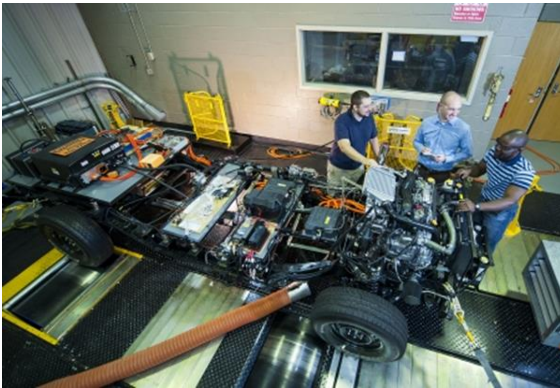
Figure 3.7 Emulator set up for testing SHEV design on Dynamometer.
